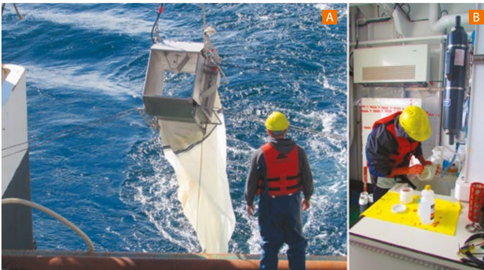
FIGURE 7. A. "Multinet". Plankton net with several cloths that open and close, allowing sampling at different depths. B. Processing of a plankton sample on board the ship.
